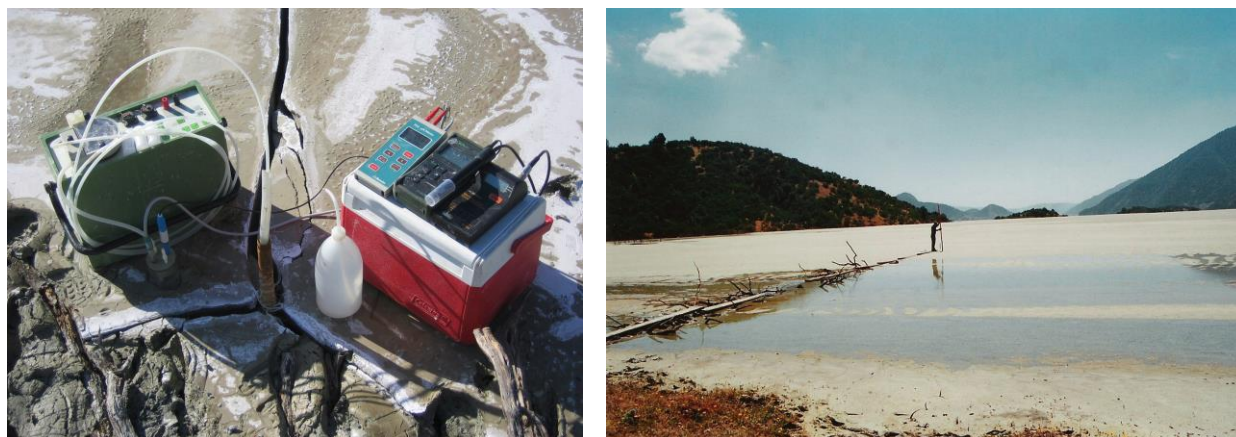
Figure 2: Sampling at point TL-26; water sampling by drive-point piezometer with measurement of pH and Eh (left picture) and sampling of tailings by a hand-corer (right picture).
